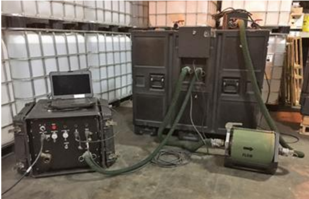
Field GDS+ (CBDS) currently fielded with SOF for field forward decontamination
