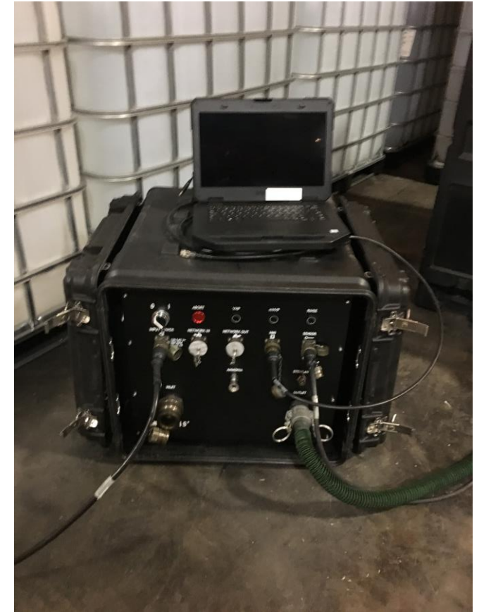
mVHP generation module can be used decontamination of rooms, vehicles or other spaces. They can be interconnected to operate in unison for larger volumes
