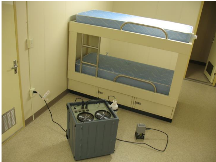
NTDS – Room vaporized hydrogen peroxide decontamination system
